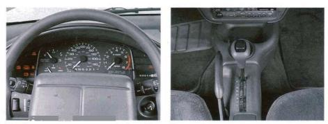
Gear indicators can be on the control panel or on the console.
