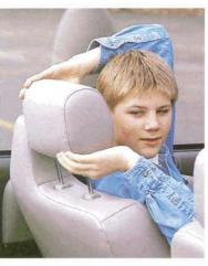
Adjust your head restraint to reach the middle of the back of the head.
