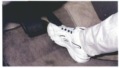
While stopped or driving in light traffic, you can try to free a stuck accelerator by putting your toe under it and lifting.
