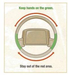
A balanced steering position between the 9 and 3 o'clock or the 8 and 4 o'clock position is best to avoid injury from an air bag.
